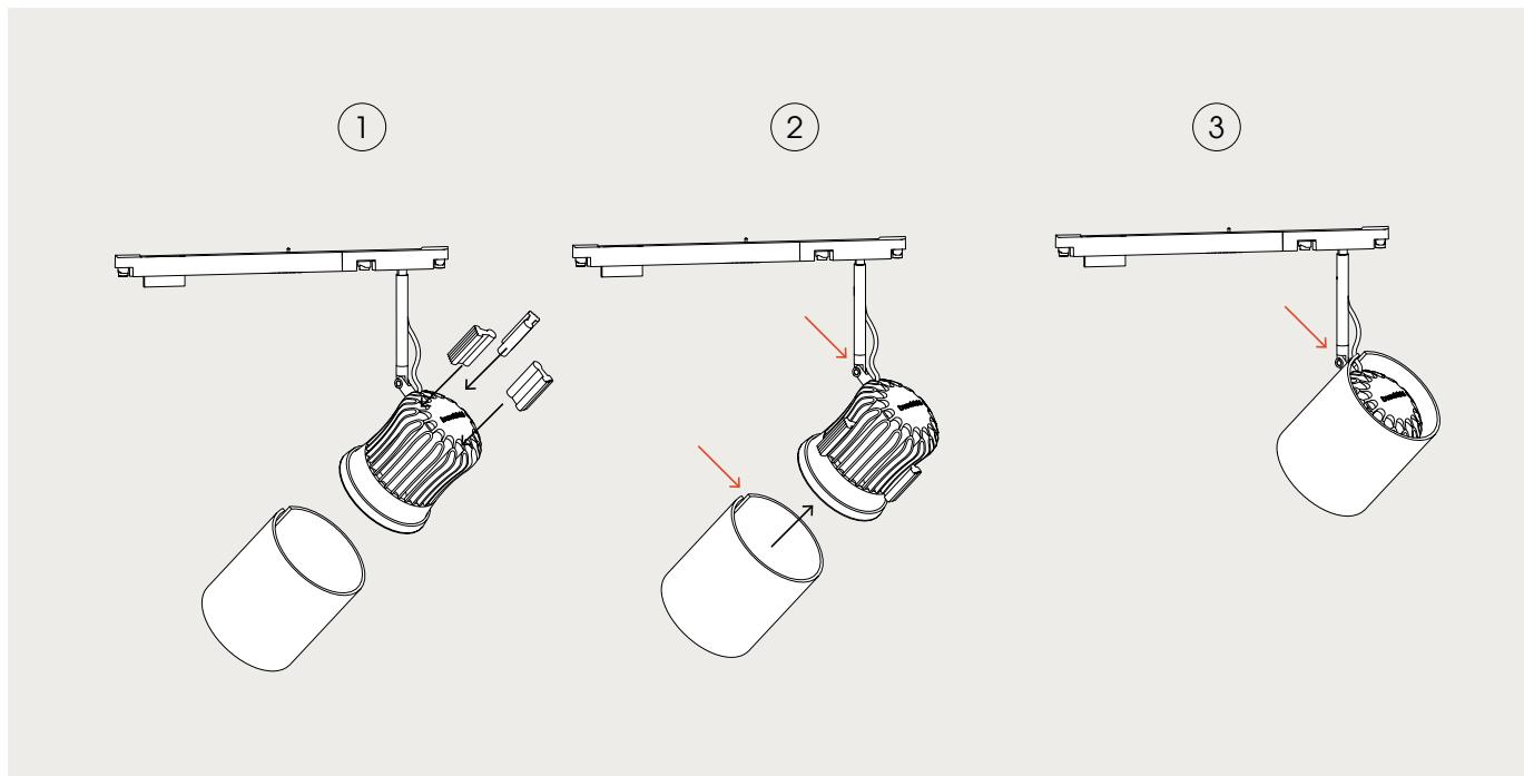
The **3 plastic holders** are inserted into the heat sink **from the rear side**. The **shade** is then slid onto the plastic holders **from the front side** of the luminaire.
