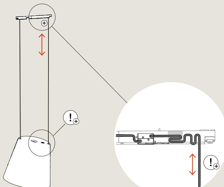
If the slight adjustment under (A) is not sufficient, the cable can be readjusted on the plus side of the adapter. To do this, unlock the luminaire and place it safely on the table. The cable length can be adjusted exactly at the marked point on the adapter. The cable is held in the adapter by the strain relief. When the cable is pushed in, it is released and can be adjusted.
