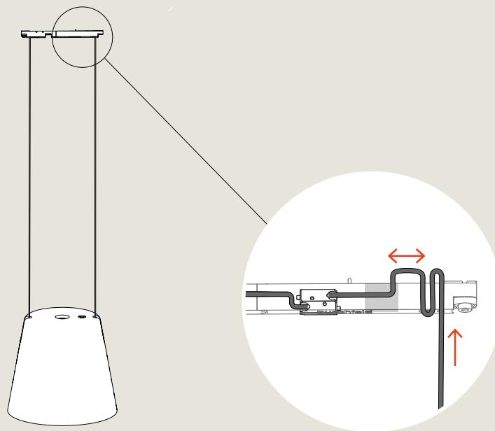
Excess cable can be pushed into the pocket in the adapter.
