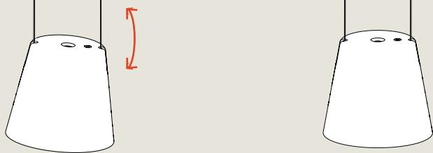
The luminaire can be straightened after insertion into the track.
